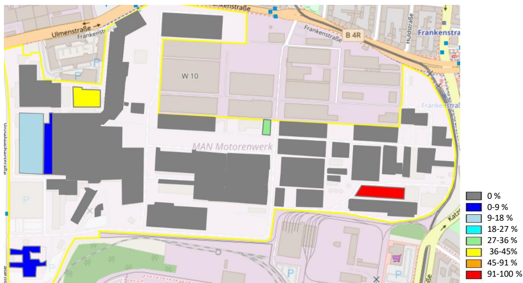
Figure 4: Standardised annual waste heat potential of the different buildings in an automotive manufacturing plant
