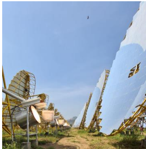
Figure 2: Scheffler Dish with static focus receiver
