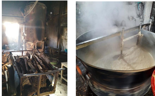
Fig. 1: Wood-fired boiler and firewood at Mahesh Khawa Kendra, Manchar, India (Source: Self-clicked) and Khoa making in-process in one of the khoa manufacturing machines (Source: Self-clicked)
