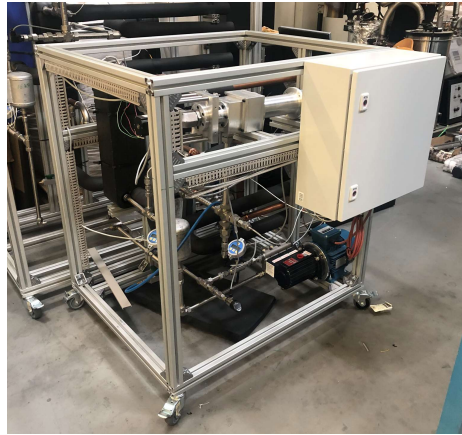
Fig. 2: Variable geometry ejector cooling system
