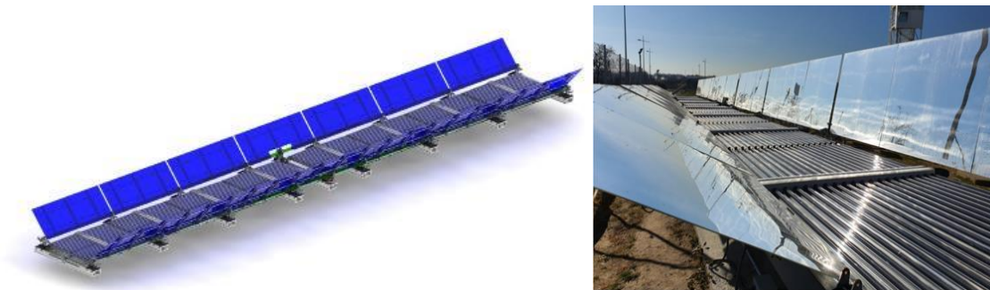
Fig. 4: WeSSun solar concentrator coupling flat sun-tracking mirrors to a fixed tilt evacuated tubular collectors
