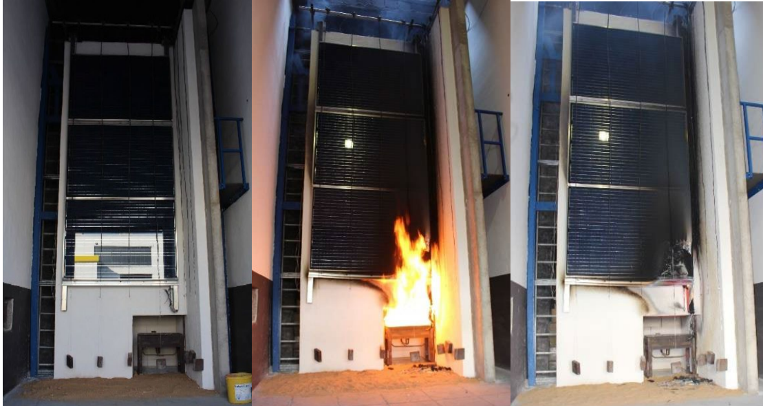
Fig. 3: Carrying out a fire test at MFPA Leipzig. Left: Before the start. Middle: During the test. Right: After distinguishing the primary burning flame
