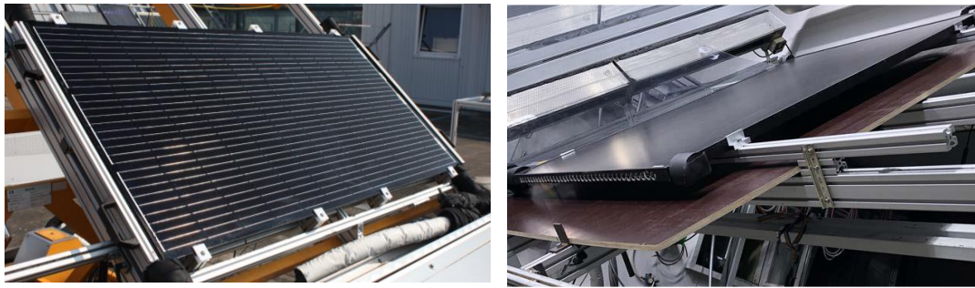
Figure 2: Collectors during outdoor (microchannel heat exchanger) and indoor (finned sheet-and-tube heat exchanger) performance testing
