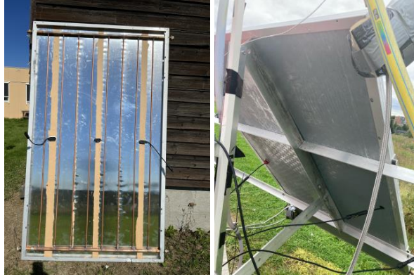
Fig. 2: Cooling loop design on the backside of the PVT module, and PVT module with insulation installed on the rack
