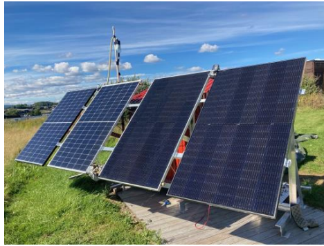
Fig. 1: Experimental setup with PERC white (PV and PVT) and PERC black (PVT and PV) modules
