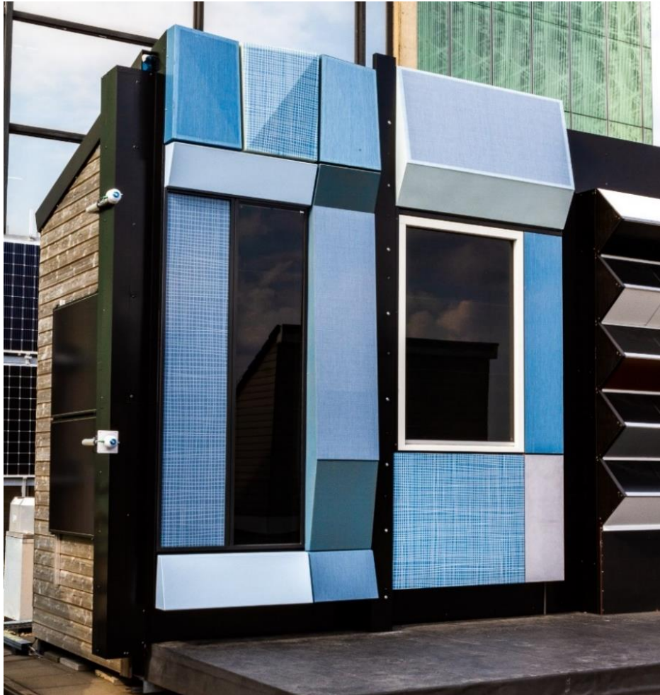
Fig. 1: PREFAB demonstrator, consisting of two façade elements, on the outdoor research facility
