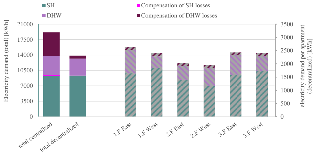
Fig. 6: Electricity demand to cover SH and DHW and the respective extra-electricity for covering losses and inefficiencies, for a centralized heating system compared to 6 decentralized systems.
