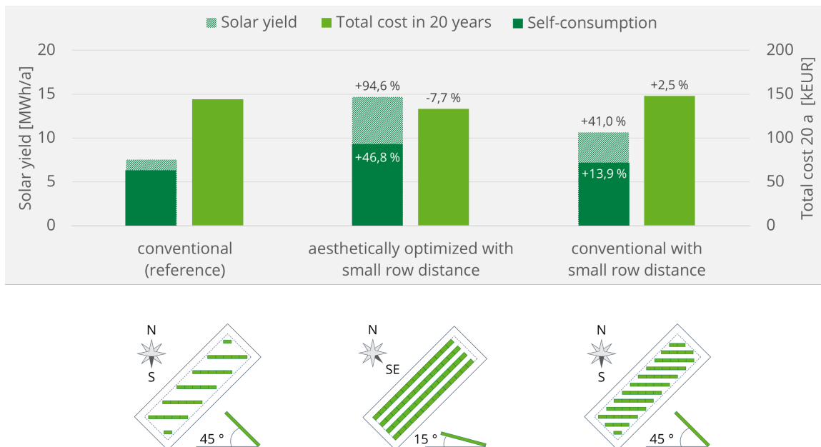
Fig. 9: Yield simulations and cost estimations for photovoltaic with reduced row distance
