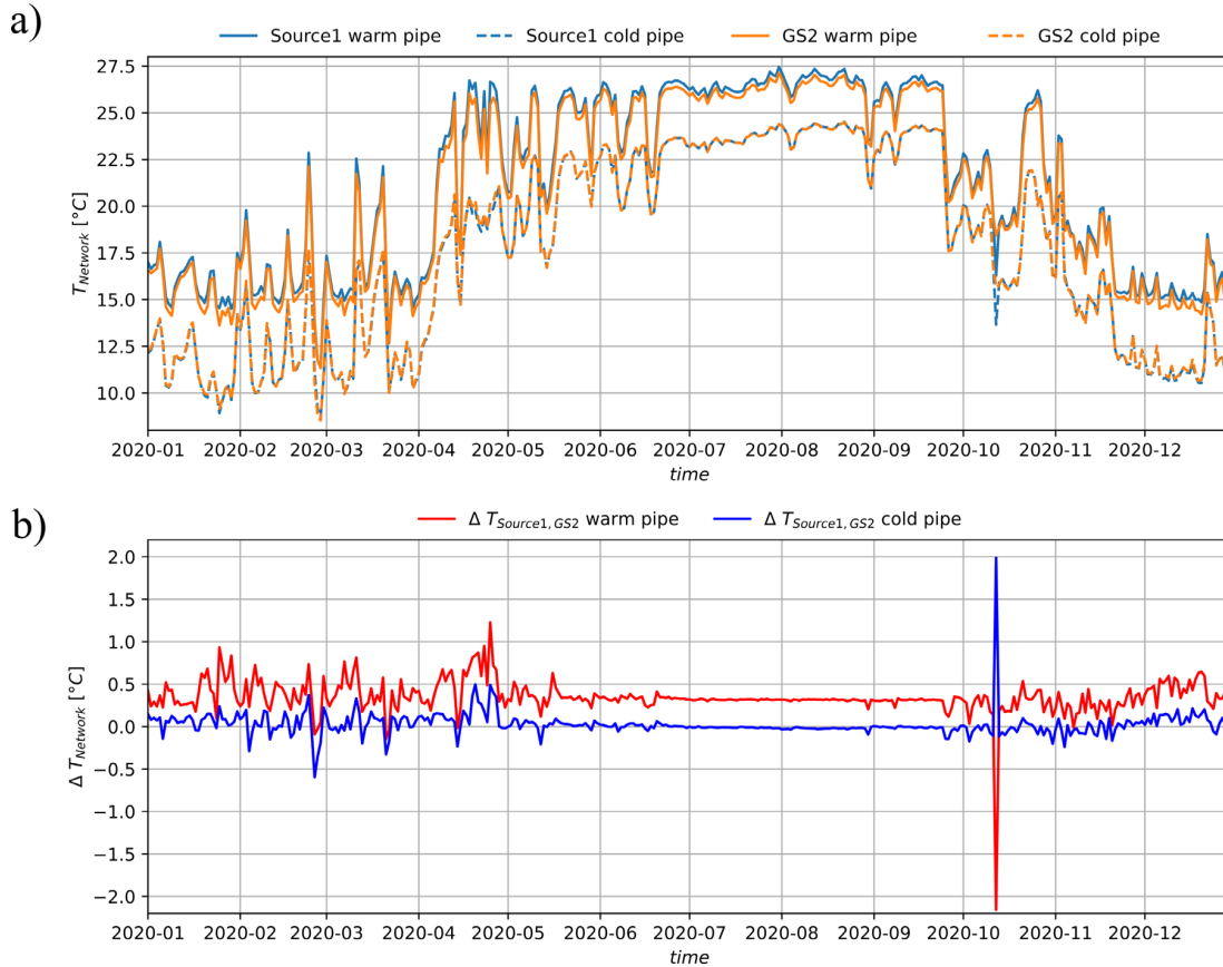
Fig. 3: a): Absolute temperature of the network for substation Source1 and Groundsource2 (GS2). The warm/cold pipes are represented by a solid/dashed lines respectively. b): Difference of network temperature between substation Source1 and GS2 for the warm pipe in red and network temperature difference between GS2 and Source1 for the cold pipe in blue. Between substations Source1 and GS2 there is 580 m of buried, uninsulated double pipe. Note that the spike in October constitutes an outlier caused by a data logging issue.
