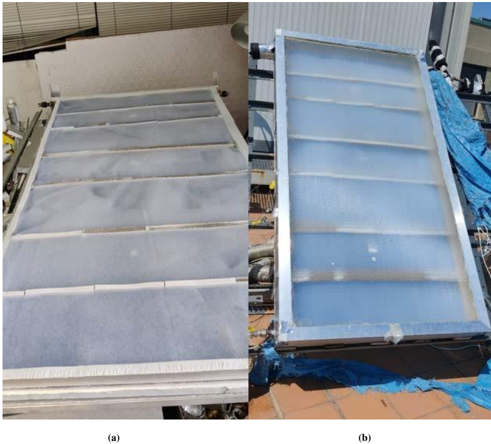
Fig. 4: Solar collector with TIM and Silica aerogel, (a) shows the silica above the absorber with a thickness of 2cm (b) represents the collector with TIM after insulation and installation.
