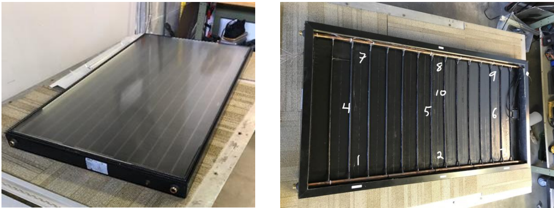
Fig. 2: Original commercial PVT collector (left) and collector being modified (right). Numbers denote the position of temperature sensors that were attached to the back of the absorber.
