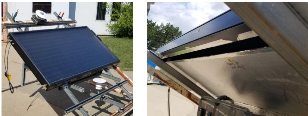
Fig. 4: Prototype undergoing outdoor stagnation testing (left), and open vent in rear of collector (right).
