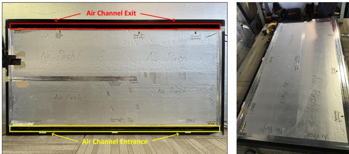
Fig. 3: Photo showing the 30 mm air channel openings installed along the full extension of the top and bottom of the collector (left, open channels), (right, channels sealed).
