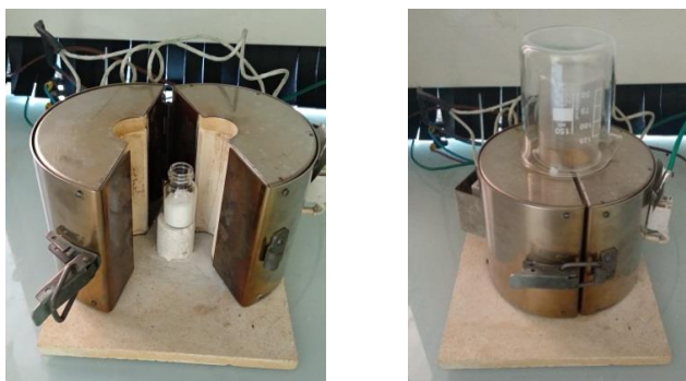
Fig. 2: Pictures of HDR oven: experimental set-up for performing thermal degradation tests.
