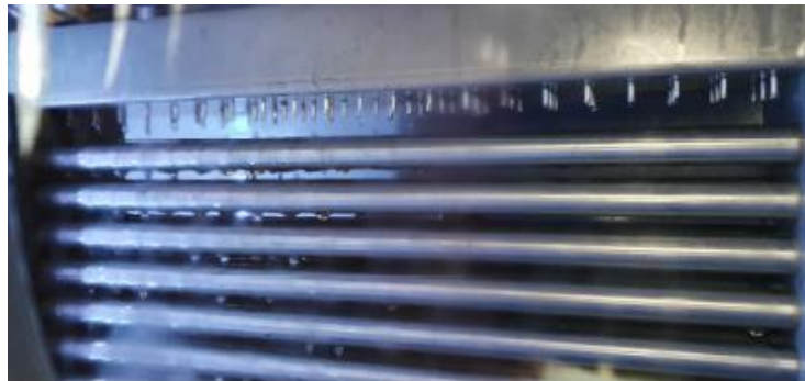
Fig. 4: Insufficient wetting of the exchange surface of the tested absorber in the experiments with a specific salt solution volume flow of \gamma = 20 l/(h·m)
