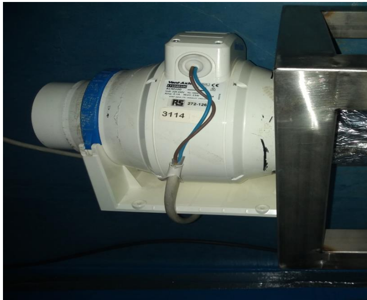
Fig. 6: Detail of the industrial air impeller located at the beginning of the tube
