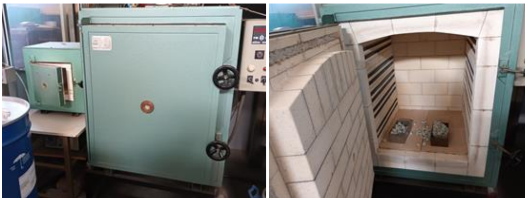
Fig. 7: Laboratory muffle furnace to dehydrate the Natural zeolite sample
