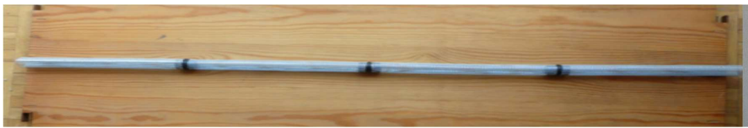
Fig. 9: Coupling of several sector cylinder condensers
