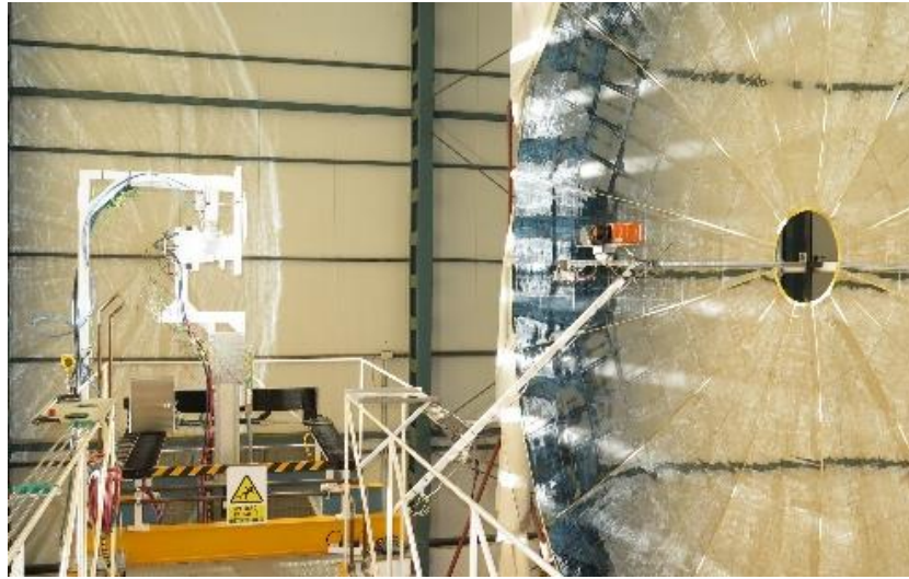
Figure 3. Accelerated ageing tests bench in solar operation at SF40.
