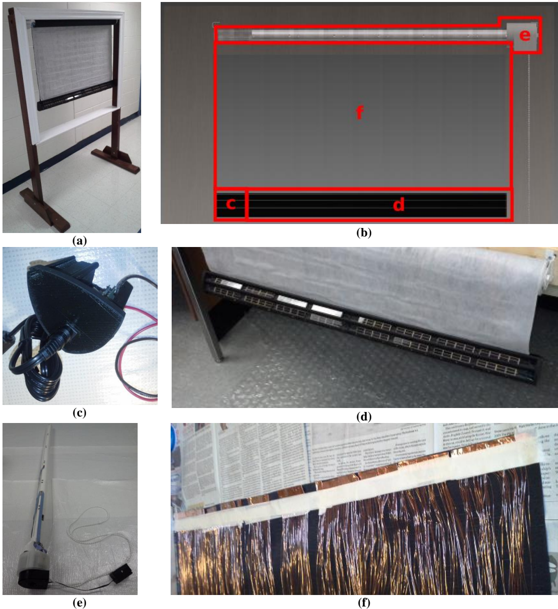
Fig. 1: Images of the prototype assembly. (a) is the entire assembled prototype. (b) illustrates the various subsystems that are shown in images (c)-(f). (c) is a backup recharging mechanism while the primary solar harvesting array is shown in (d). The electronics that operate the window blind are shown in (e). The solar array and control electronics are connected through conductive fabric shown in (f).
