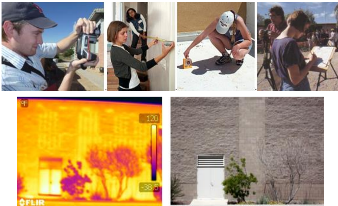
Fig. 13: Above, auditors using thermal camera, measuring internal dimensions, roof tilt and sketching facades, Below: An infrared photo showing the CMU wall with thermal bridges through the grout
