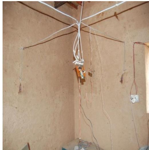
Fig. 10: Adobe building with sensors connecting to a transmitting module
