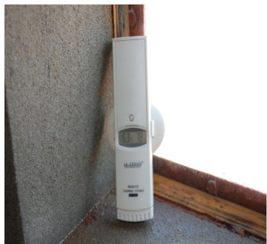
Fig. 12: Sensor inside brick building to monitor inside temperature and humidity.
