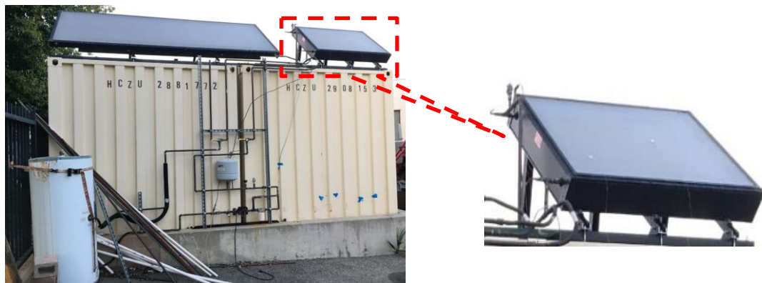
Fig. 2: Experimental test set-up for ICS system
