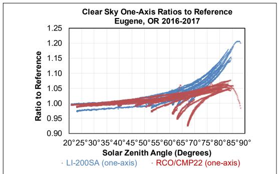
Fig. 6: Clear-sky ratio data between a LI-200S pyranometer and a RCO reference cell against the reference CMP 22 pyranometer. Clear-sky periods were shown for each month of the year.
