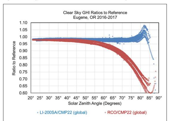
Fig. 3: Ratio of a LI-200SA pyranometer (blue triangles) and RCO reference cells (red circles) values divided by the values from the reference CMP 22 pyranometeer on a horizontal surface during clear skies for selected days throughout the year at Eugene, Oregon.
