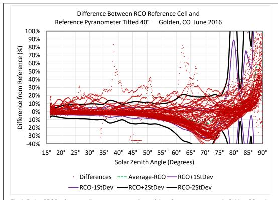
Fig. 9: Ratio of RCO reference cell measurements to those of the reference pyranometer in Golden, CO under all weather conditions in June, 2016. The dotted green line shows the average value and the thin purple lines show one standard deviation from the average. The thick black lines show the two standard devations from the average. Ninety five percent of the data points should be within two standard deviations for a Guassian distribution of the differences.
