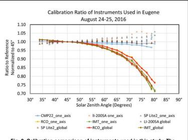
Fig. 2. Calibration comparison of instruments used in this study. The responsivities at 45° are used to normalize the calibrations.
