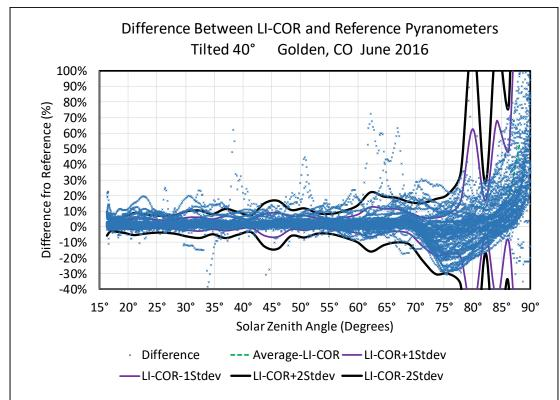
Fig. 8: Ratio of LI-200A measurements to those of the reference pyranometer in Golden, CO under all weather conditions in June, 2016. The dotted green line shows the average value and the thin purple lines show one standard deviation from the average. The thick black lines show the two standard devations from the average. 95% of the data points should be within two standard deviations for a Guassian distribution of the differences.
