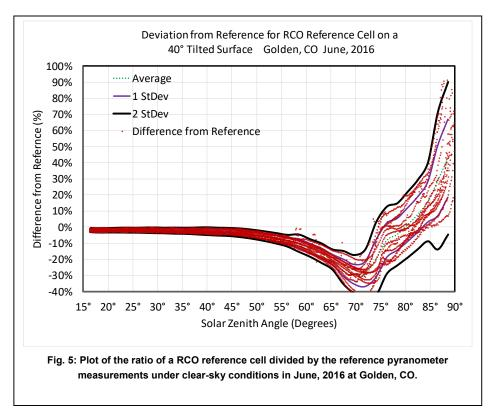
a horizontal surface at an SZA of 65°. The reason for the increased deviance is that the angle-of-incidence is greater than in the horizontal case. In fact, at an SZA of approximately 75°, the sun is setting behind the tilted surface. The spectral distribution of the ground reflected irradiance also plays a role. The magnitude of the spectral distribution effects will be the subject of a future paper.
