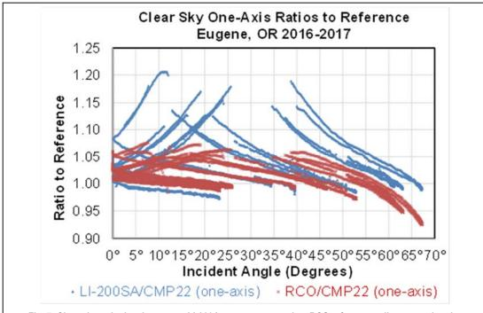
Fig. 7: Clear-sky ratio data between a LI-200A pyranometer and an RCO reference cell compared to the reference CMP 22 pyranometer plotted against the incident angle instead of SZA. Clear-sky periods are shown for each month of the year.
