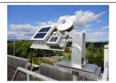
Fig. 1: Pyranometers and reference cells on a one-axis tracker in Eugene, Oregon.
