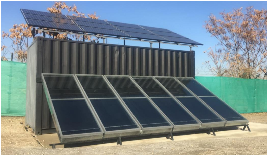
Fig. 14. Modern commercial scale indirect solar food dryer in central Afghanistan with active fans for large scale food drying increases production and reduces spoilage.
