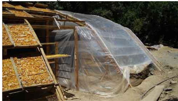
Figure 3. Direct greenhouse dryer used by the French NGO GERES in Afghanistan for apricots.
