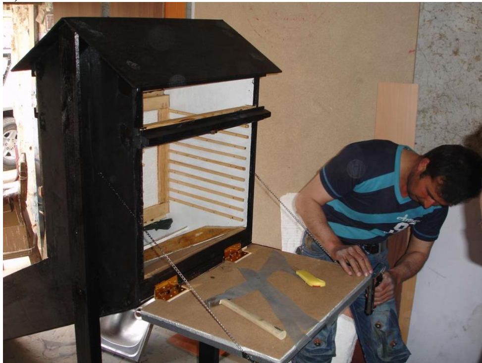
Figure 5. NMSU trained Afghan carpenters such as Mr. Hakim on how to build indirect solar food dryers using all local materials.
