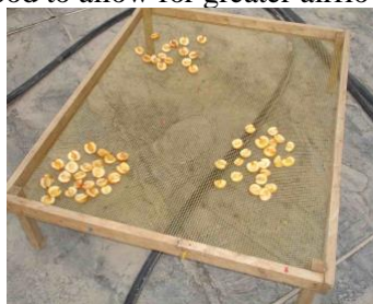
Figure 2. Outdoor rack type dryer drying apricots in Afghanistan which allows for better air circulation underneath the product.
