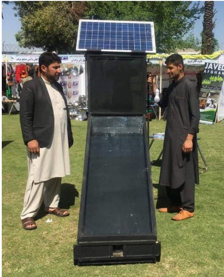
Figure 13. Indirect solar dryer innovation in 2021 by Zaib Pamir Co. with the addition of an active fan powered by a PV module to increase drying rates and productivity.
