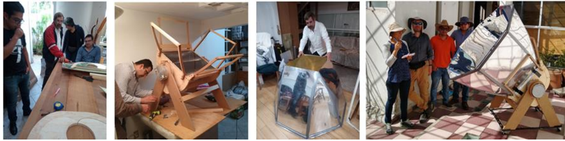
Fig. 10: Artisanal construction of the first prototype of the Tolokatsin 2020 solar oven
