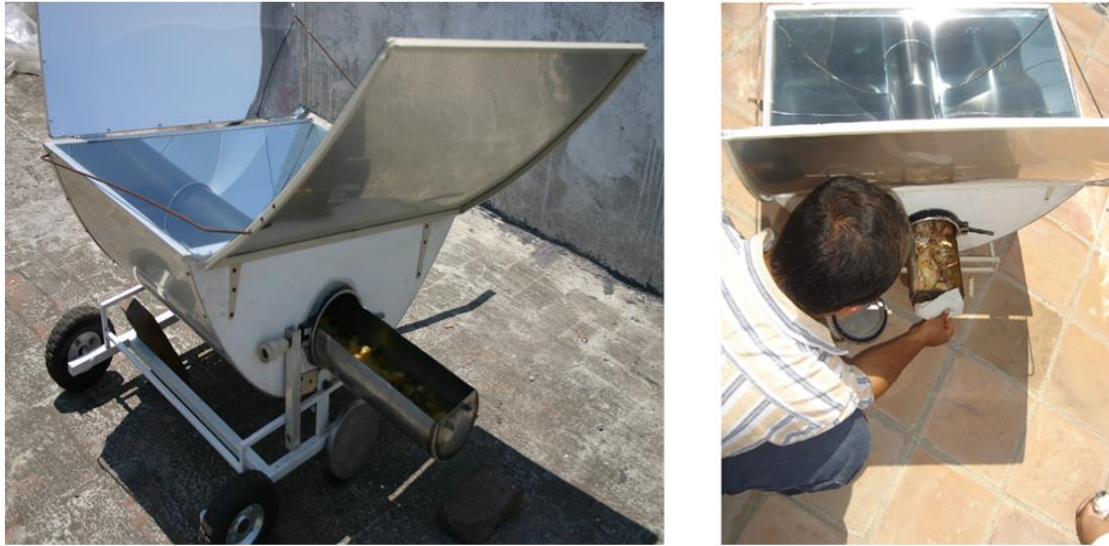
Fig. 6: Photographs of two Tolokatsin solar cookers model 1995 with their containers opened showing their stainless steel trays with cooked meals inside them
