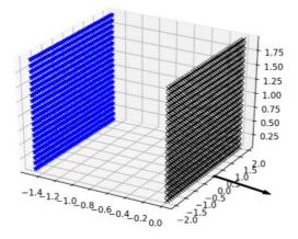
**Fig. 4:** Geometry for demonstrations of combined shading, reflection, and irradiance analysis. Each of the collector (right) grid points are marked with an X and stars mark the grid points of the reflector (left). The arrow to the right points south.
