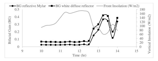
Fig. 10: Experimental data for side by side vertical modules simulating bifacial panels enhanced with a Mylar white diffuse reflectors compared to a monofacial panel on July 9, 2021.
