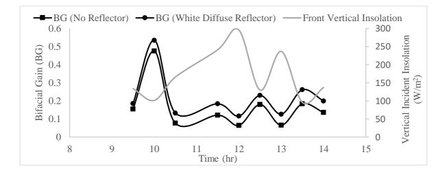
Fig. 9: Experimental data for side by side vertical modules simulating bifacial with no reflector and one enhanced with white diffuse compared to a monofacial panel on July 15, 2021
