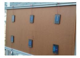
Fig: 2: a) 3D rendering of the orientation for the second experimental setup and image of b) photovoltaic cells simulating different positions on the rear side of a collector
