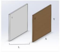
Fig. 1: Geometry for parallel surface view factor where i is the reflector and j is the collector.
