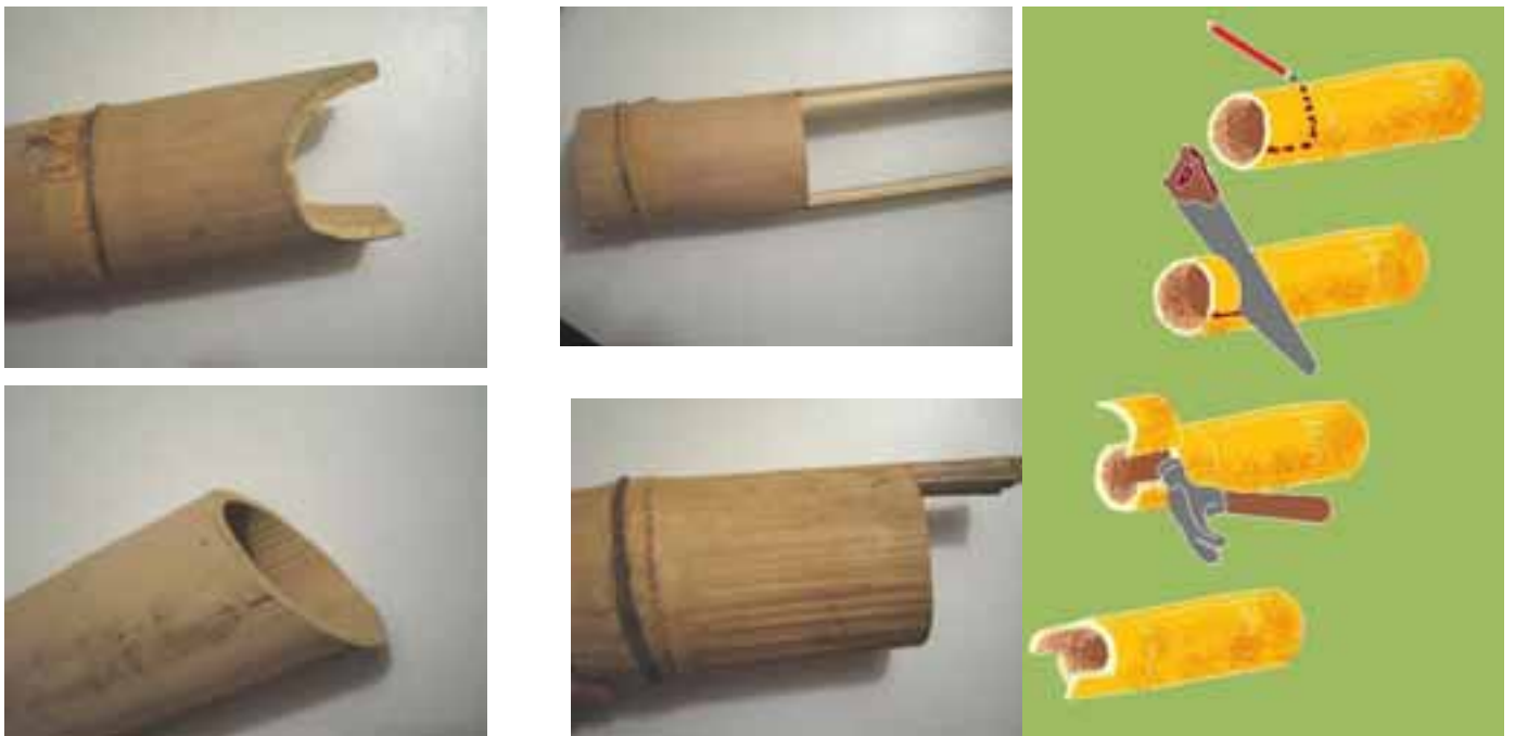
Figure 4 the basic bamboo cuts, also exist variation of each one to the accommodation for building construction.
