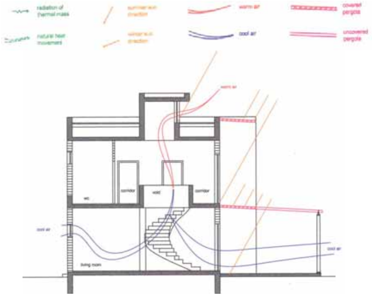
Figure 2.2 winter design considerations (north-south section through the staircase)
