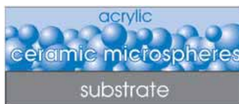
Figure 2 – Paint film with ceramic microspheres (Paint Quality Institute, http://www.paintquality.com/ ) .
