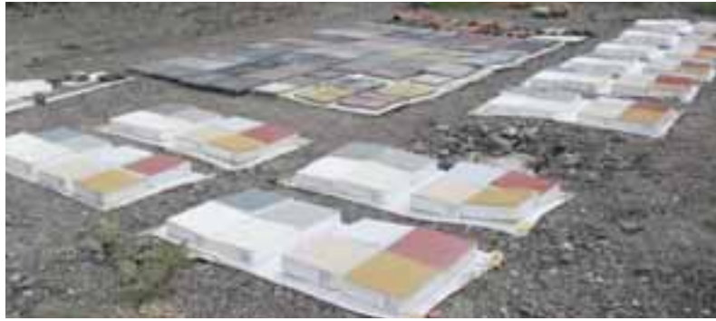
Fig. 2: Thermal and optic evaluation of the materials on site.
