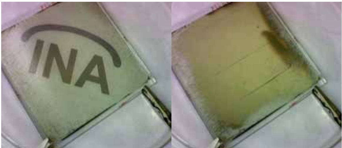
Fig. 13: Electrostatic actuation of the micro mirrors: a module with micro mirrors in their open state, without any voltage applied (left) and in their closed state with a voltage of 80 V applied (right)
