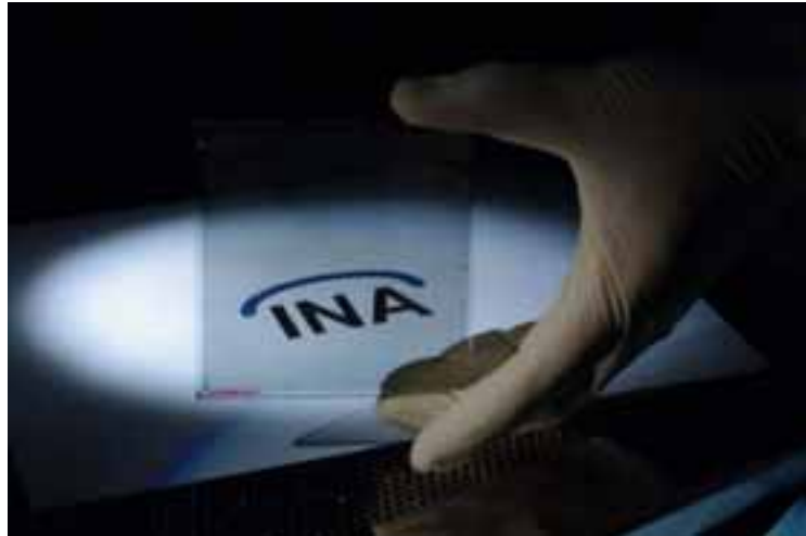
Fig. 10: Micro mirror array – module with a size of 10cm x 10cm
