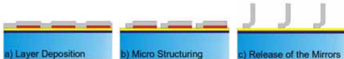
Fig 3: Basic fabrication steps of the micro mirror arrays
