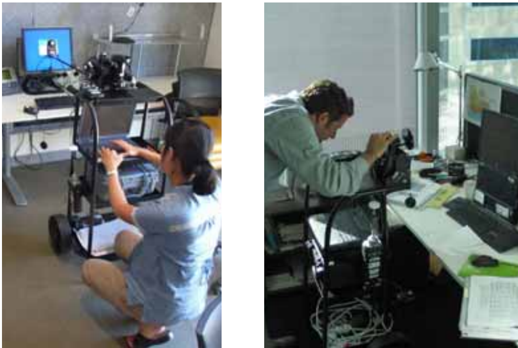
Fig.2 Showing the 'Visual Comfort Meter' in illuminance (left) and luminance (right) measurements.
