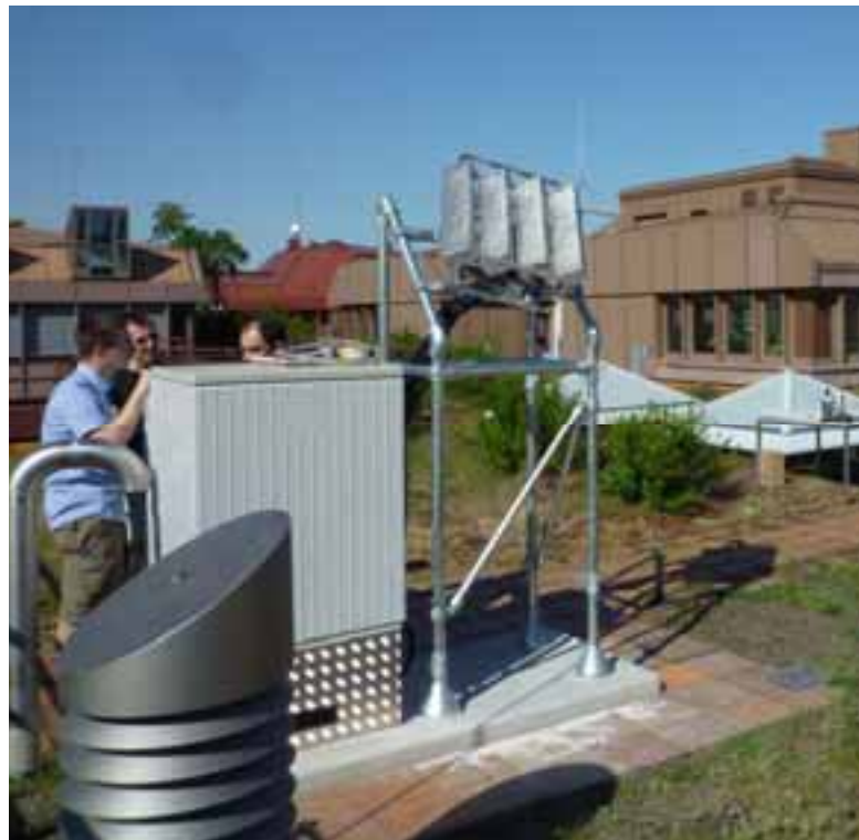
Fig. 7: Current version of Sollektor with 8 fiber bundles carrying 108 individual POF each
