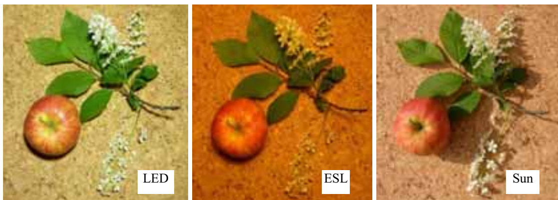
Fig. 5: Different colour rendering using different light sources; all photos taken with identical camera setting
