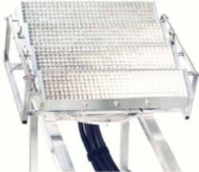
Fig. 6: Current version of Sollektor with 8 fiber bundles carrying 108 individual POF each
