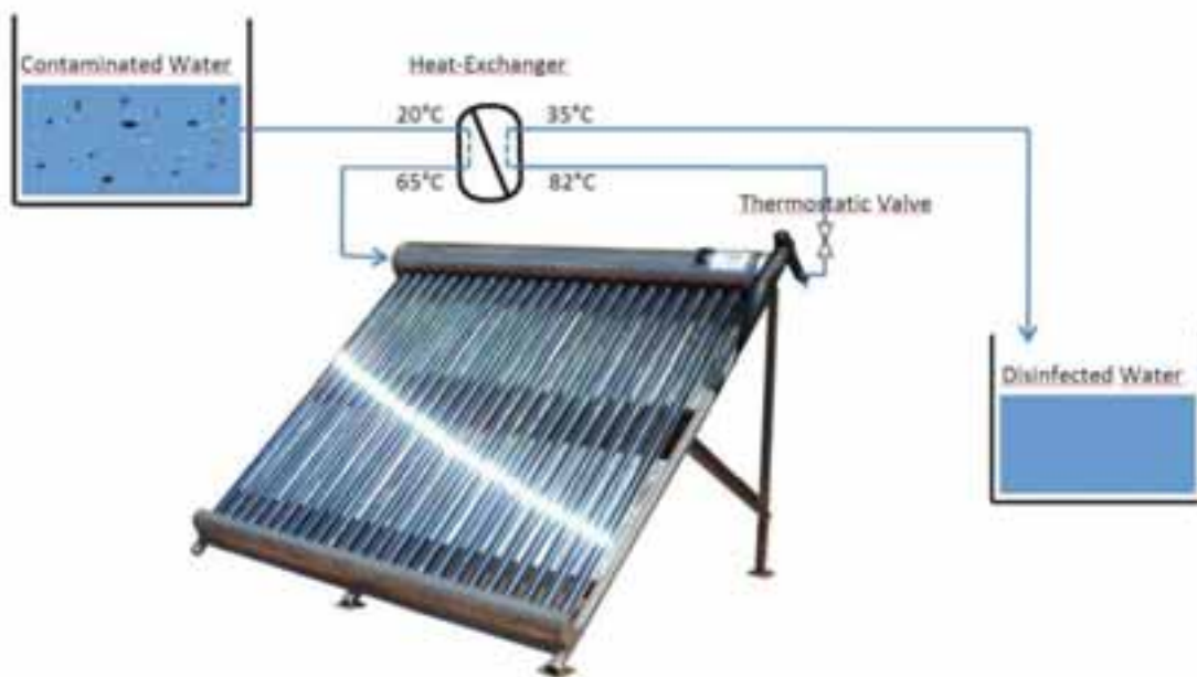
Fig. 1: Scheme of the solar thermal pasteurization plant with its main components heat-exchanger, collector and thermostatic valve (adapted from Konersmann and Frank, 2009). General functionality is indicated in the text box on the right.
