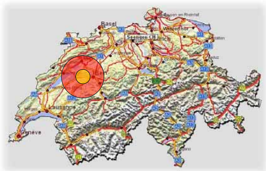
Fig. 4: Yellow: area needed to produce the total amount of consumed electricity using photovoltaic in Switzerland (60 TWh). Red area: 30 km circle similar to the Fukushima evacuation zone.
