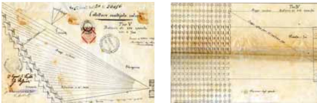
Fig. 3: Drawings from Battaglia’s “Collettore multiplo solare” patent. Left, Cross section of the collecting reflector area and the longitudinal grounded boiler, one meter in height, installed inside a brick oven, insulating and protecting the boiler and with an opened window facing the reflector area. Right, Plan of the collecting reflector area and of the longitudinal or linear boiler, roughly ten meters in length. (Drawings, Central State Archive, Rome, Italy).
