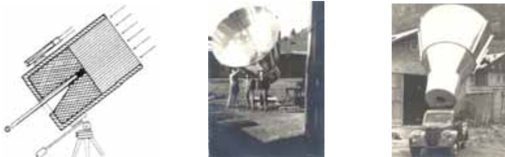
Fig. 5: Left: first honeycomb absorber that Francia built in 1960; Right: Photos of the first boiler coupled with a concentrator and protected by a honeycomb structure tested in Cesana Torinese in 1960/1961. To track the sun the boiler was moved by a small truck (photos 1960, Francia Archive, MUsl Brescia).
