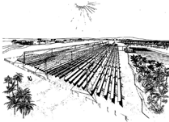
Fig. 9 – Artist’s rendering of an LFC solar power plant designed by Giovanni Francia and collaborators in the late 1970s (Ansaldo Meccanico Nucleare, 1980).
