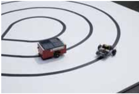
Fig. 91: SolaRobots following the line
