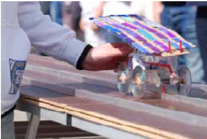
Fig. 7: Selfmade vehicle with a lot of recycling material, e.g. wheels from CD's
