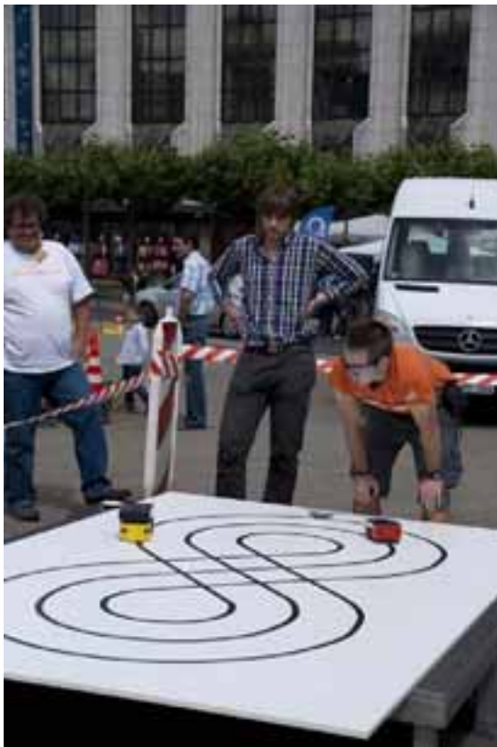
Fig. 80: SolaRobots following the line conducted by a micro-controller
