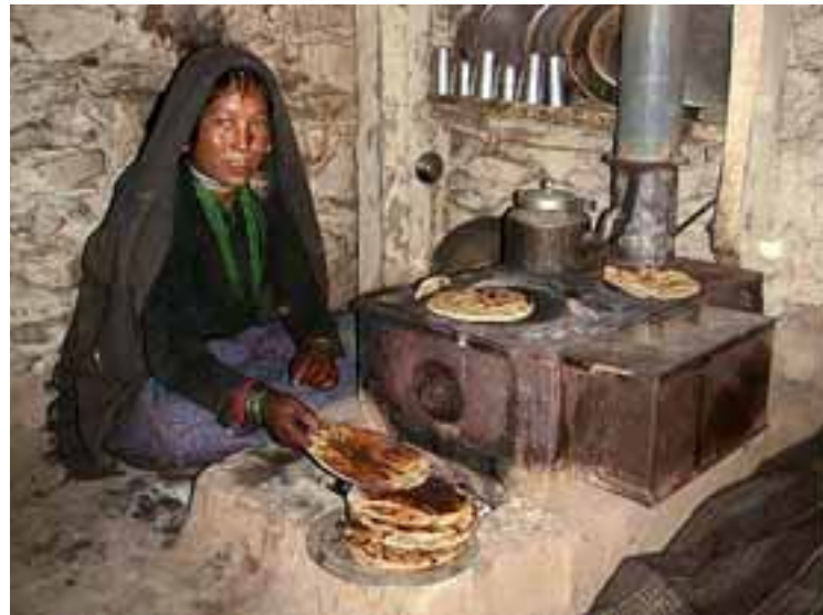
Fig 3: The Smokeless Metal Stove (SMS) which I designed in 1998, has been continually improved. Up to the end of 2010 over 5,000 homes in the remote districts of Nepal have had one installed. It cooks the traditional food “dhal bhat” all at one time and “roti”, uses ~40% less firewood, provides appropriate room heating and 9-litres of hot water for drinking the local “butter tea” as well as facilitating an improvement in personal hygiene. This is called “contextualised” technology, with people, their culture and way of living in the centre and technology developed to suit them in their context.
