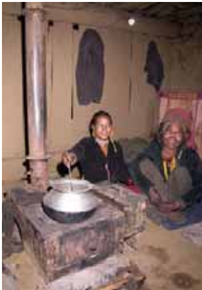
Fig 2: Alongside the efficient smokeless metal stove, designed for the particular local cooking culture and heating needs, also WLED lamps for minimal but locally appropriate, long-lasting light services, are installed in each home, as part of the “Family of 4” HCD concept.
