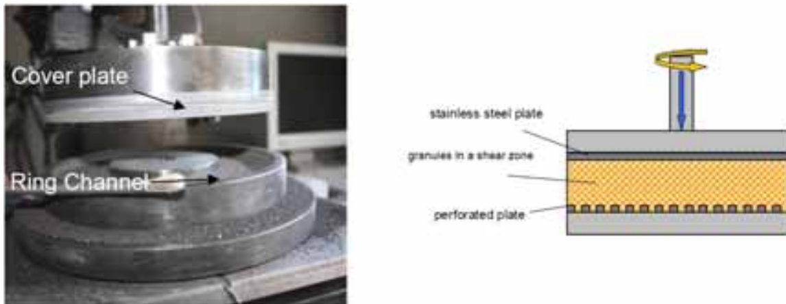
Fig. 6: Shear cell device (left), principle of the shear cell (right)
