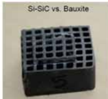
Fig. 8: Re-SiC after abrasion by basalt (left) and Si-SiC after abrasion by bauxite (right)
