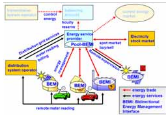
Fig. 10: Possible interaction of the energy management system Pool-BEMI/ BEMI
