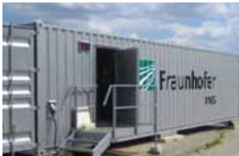
Fig. 10.1 and 10.2: Mobile MV LVRT container (left picture) and simplified schematic of the LVRT container according to FGW TR3 (right picture) with measuring points MP1 to MP3, decoupling / short-circuit impedances Z_G , Z_1 and Z_2 and switches / circuit breakers S1 and S2
