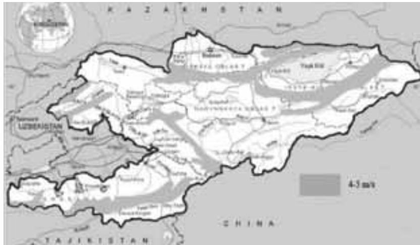
Fig.6 : The wind potential of the Kyrgyz republic (Master Plan of Wind Power Development of the USSR 1989)
