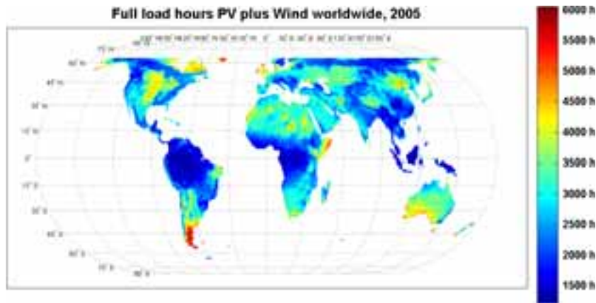
Fig. 4: Full load hours of fixed optimally tilted PV power plants (top, left), of wind power plants of 150 m hub height (top, right) and of hybrid PV and wind power plants (bottom). Calculations are performed for all hours of the year 2005 and all coordinates of a 1°x1° mesh of latitude and longitude within 65° N/S.
