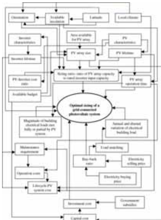
Fig. 6. Interactions of influences on PV system sizing (Mondol et al, 2005)
