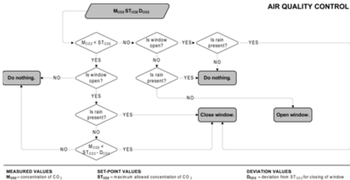
Fig. 5: Flow chart illustrating the functioning the air quality control of the ICsIE.
