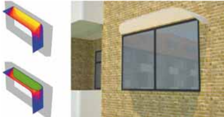
Fig. 2: Illustration of the design of the fixed solar shading showing insolation intensity and minimization of surface area (left) and the final geometry added to the existing façade (right)
