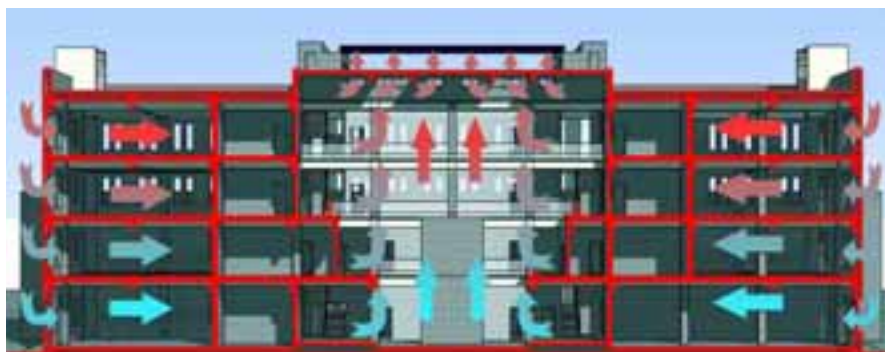
Fig. 3 Summer Ventilation Diagram
