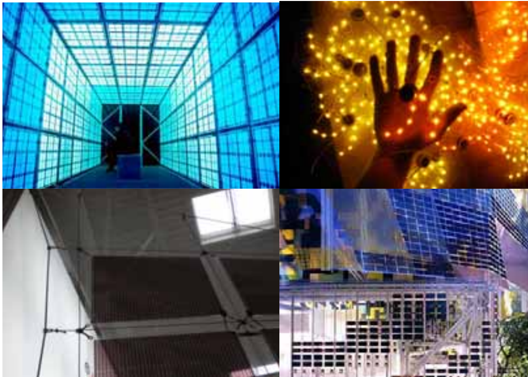
Fig. 10: (top left) Boxenstopp , Branschweig (D), Daniel Hausig, 2000. The envelope is made of, outside, solar cells and electroluminescent cells from inside (pictures: C. Luling) (top right) "Metabolic Media." Synthetic textile with micro LED powered by flexible organic solar cells or DSC. The traditional surface becomes dynamic, bright screens. (Photo: www.loop.ph ) (bottom left) Solar Tensile in Intersolar 2011 Monaco; (bottom right) "Wrap @ Smart". Research by Stefan Kieran and James Timberlake Architects, 2003. Testing of innovative building multifunctional composite material. The printed thin film solar cells, storage energy and, in combination with OLED technology, enabling the lighting of the interior, where the phase change materials provide to microclimate control. (Photo: www.kierantimberlake.com )
