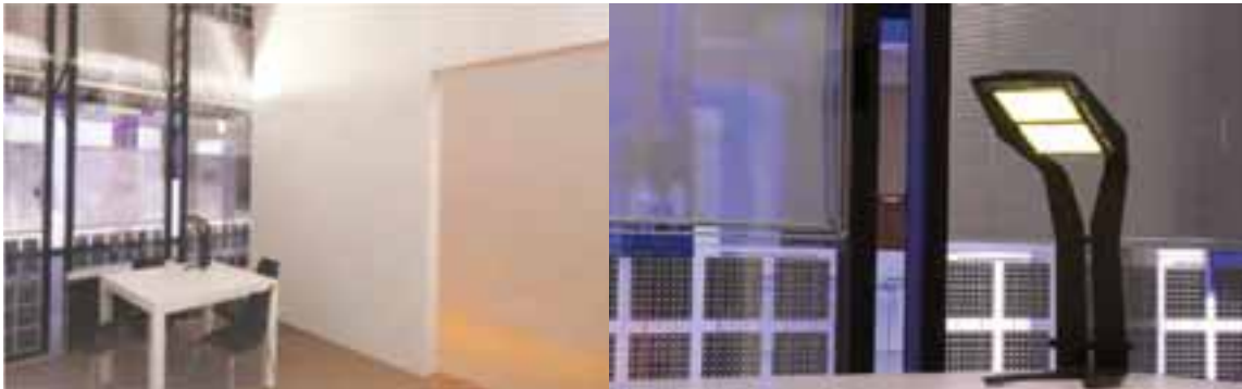
Fig. 9: "Future Cube". Concept design of multifunctional solar facade able to perform complex functions, such as solar control, the spread of natural light, artificial lighting, aeration and ventilation. Collaborative project developed by Behnisch Architekten, Zumtobel Lighting, Transsolar Energietechnik, Sunways, Bartenbach Lichtlabor, 2010 (images: The Plan).
