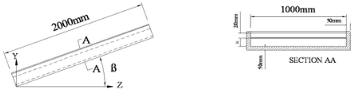
Fig. 2. Collector orientation and dimensions considered for simulation
